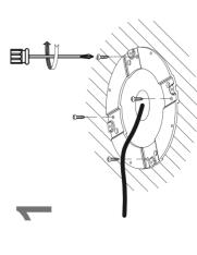
This light can be fitted on concrete, wooden decking or by using a ground spike. see the next 2 pages for details how to assemble each option.
